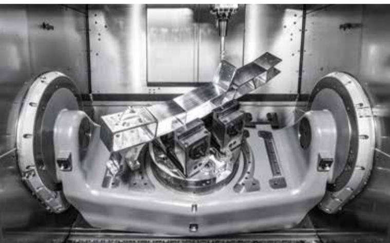
The large working area of the C 42 U machining centre, with three axes in the tool (X-Y-Z) and two axes (C and A - 440 mm swivelling rotary table) in the workpiece for optimal tool deployment during 5-axis full / simultaneous machining of complex aerospace components
