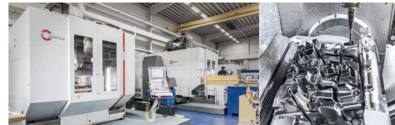
left The new C 52 U five-axis machining centre right Working area of the C 52 U with the 700 mm swivelling rotary table capable of bearing 2000 kg; equipped here with a large scale base tool being finished in 5 axis operation
